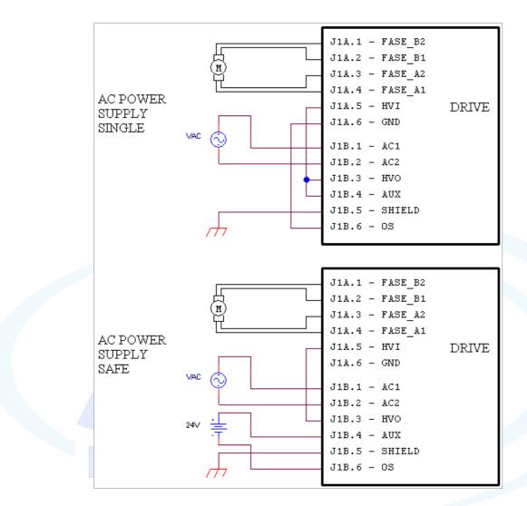
In AC power mode do not connect GND signals between two or more HT7 drives:
